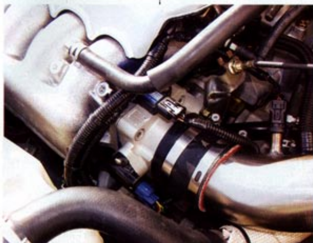
We bolted on a K20 intake manifold from a Japanese RSX Type-R, 68mm billet throttle body and custom intake.
