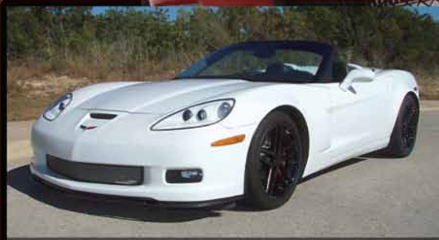
LS2, ProCharger F-1C, 8-rib Drive System, 16.5 psi, 905 RWHP
