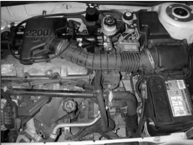
a. Factory air box system installed.
