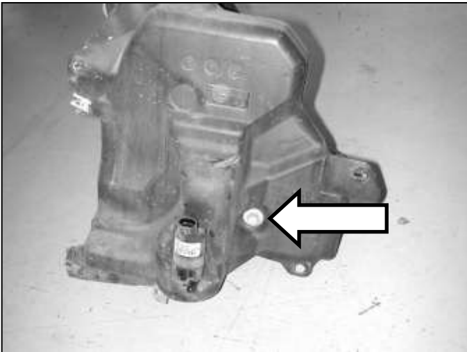
q. Remove the washer bottle from the vehicle. Loosen the bolt connecting the bottle to the lower air box.
