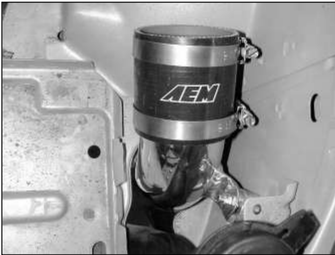
f. Install the supplied silicone hose as shown. Orient the hose clamp screws away from the battery tray as shown.
